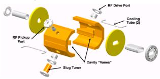
Figure 5: Exploded view of the 500MHz RF kicker cavity showing the vanes.
