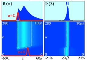
Figure 7: Final, steady-state optical pulse shape E(z) (bluetop left) for 120λ, with the electron pulse (red) superimposed at z=L. The relative positions at z=0 (bottom left) shows the electron pulse a full 30\lambda ahead of the optical pulse. The intensity (bottom left) and spectral (bottom right) evolution of the optical pulse shape (light blue) is shown over the n=280 amplification passes of the 10 µs macropulse. The final optical spectrum  $P(\lambda)$  has an ~2.5% width (top right).
