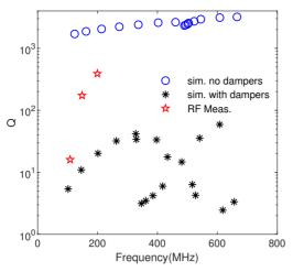
Figure 4: Simulation results of quality factors of the trapped RF modes in the IVU with and without ferrite dampers.
