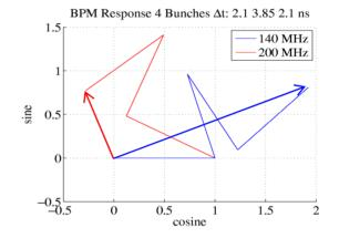
Figure 6: Vector addition of four BPM signals for different frequencies. The typical Linac BPM with 140 MHz (blue) shows about a factor of two (2.06) of the single bunch charge for the sum of four bunches, while an LTU (Linac To Undulator) BPM (red) shows with 73 % less than a single bunch. Four different types of BPMs are used along the accelerator (top).
