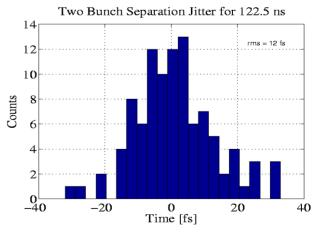
Figure 2: Two-bunch timing separation jitter measured by looking at the bunch separation on the dump screen (top) which is used together with the transverse deflection cavity XTCAV.
