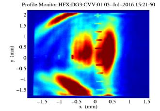
Figure 1: Profile monitor screen 270 m downstream of the K-Mono. The first bunch is where the two central lopes are (from the old, non-prefect mirrors). The second bunch is from pulse to pulse very different and here on a part of a circle which is already outside some collimation jaws.
