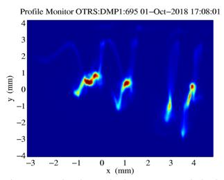
Figure 5: Four bunches on the dump screen. Vertical axis is energy, horizontal is time. From right to left is L2B1 (Laser 2 Bunch 1), L2B4, L1B1, L1B4. B4 has a short bunch length and is close to B1 for L2, while B4 is long and further behind for L1, although they go through the same de-
