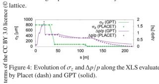
Figure 4: Evolution of  $\sigma_z$  and  $\Delta p/p$  along the XLS evaluated by Placet (dash) and GPT (solid).
