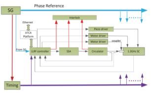
Figure 2: RF station architecture.
