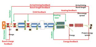
Figure 8: The layout of the injector feedback system.
