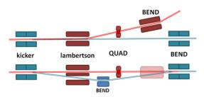
Figure 7: The layout of the beam distribution system.
