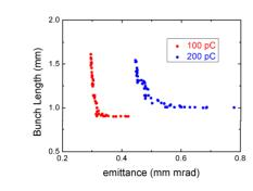
Figure 2: Multi-objective optimization results of the injector.
