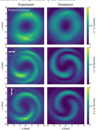
Figure 3: Obtained intensity distributions in experiment (left column) and simulation (right column). Top row shows intensity without polarizer. Middle and bottom rows show intensity through horizontally and vertically oriented polarizer.
