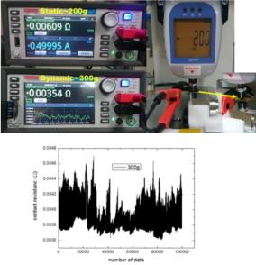
Figure 6: The top figure shows the experimental equipment and the lower graph shows the measured data when the devices are in continuous dynamic motion.
