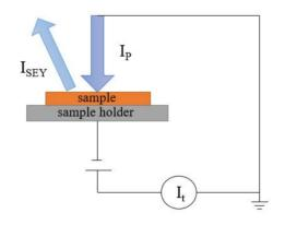
Figure 1: Schematic diagram of the SEY measurement.
