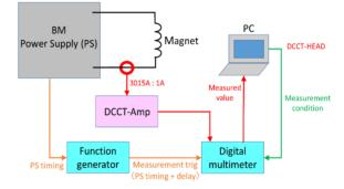
Figure 1: Configuration of the measurement system.
