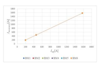
Figure 4: Linearity of reference current and measured current.
