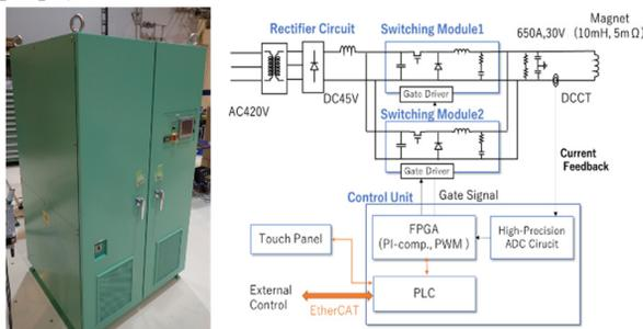
Figure 6: Picture (left) and schematic diagram (right) of the high power PS.
