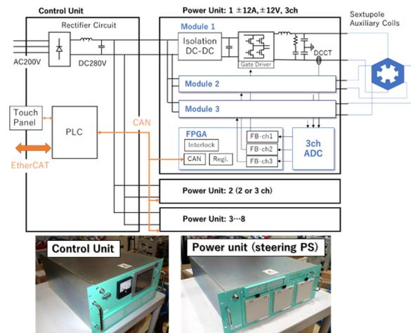
Figure 7: Schematic diagram (upper) and pictures (under) of DC-link PS system.
