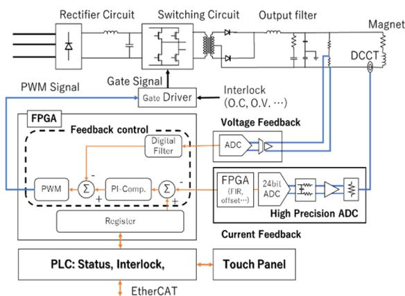
Figure 1: Schematic diagram of an overview of digital feedback system.
