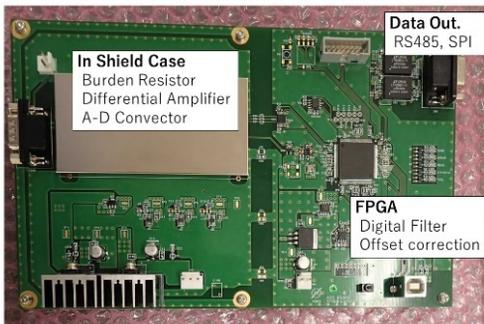
Figure 2: Overview of high precision ADC circuit.
