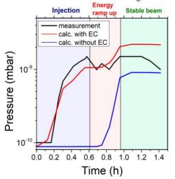
É Figure 5: Time evolution of pressure during the fill 7319: measurements (black line), results of the DYVACS simulation with the electron cloud (red line) and without the electron cloud (blue line).
