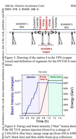
Figure 4: Energy and beam intensity ("blue" beam) during 2.85x1014, blue line), energy ramp up (from 450 to 6500 GeV, black line) and then stable beam (p-p collisions).
