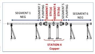
Figure 3: Drawing of the station 4 in the VPS (copper vessel) and definition of segments for the DYVACS simu-
