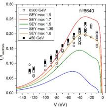
© Figure 4: Variation of I<sub>+</sub>/I<sub>electrons</sub> vs V<sub>bias</sub>: experimental data
