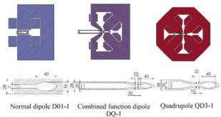
Figure 3: Cross-section of stainless steel vacuum chamber inside magnets. The machining and positioning of the bending chamber must be precise for not to conflict with the active components nearby.
