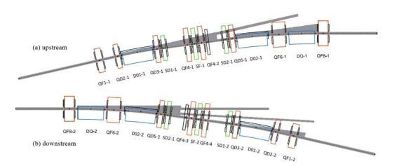
Figure 2: Top-view layout of the upstream (a) and downstream(b) chambers inside the DTBA cell magnets.
