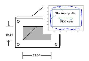
Figure 2: WR90 waveguide geometry showing location of NEG sputtering wires and resulting theoretical thickness profiles.
