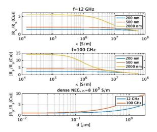
Figure 1: Analytically calculated surface impedance of thin NEG coatings on copper substrate normalized to uncoated copper: variation with conductivity and coating thickness.
