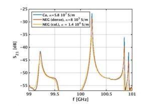
Figure 6: Calculated transmission between waveguides, the 2 TEM<sub>0,0,38</sub> resonance sits at 100.2 GHz.
