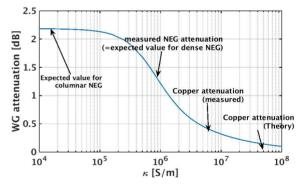
Figure 4: Calculated attenuation and conductivity together with known data points.
