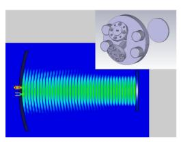
Figure 5: Field distribution of Fabry Perot including 3D structure.
