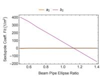
Figure 4: Sextupole coefficients  $a_2$  and  $b_2$  versus beam pipe ellipse shape.
