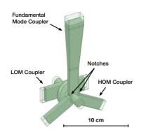
Figure 5: Elliptical crab cavity with the input, LOM, and HOM couplers.
