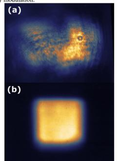
Figure 3: UV laser image measured at the virtual cathode (a) is taken without MLA, and (b) is taken with MLA.
