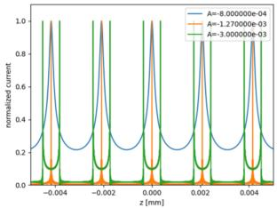
Figure 2: Estimated current profile after the EEX beamline with given transverse modulation amplitude *A*.
