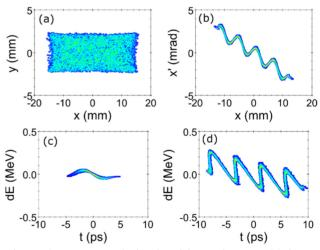
Figure 4: Start-to-end simulated beam images. (a) beam image at the entrance to the transverse wiggler. (b) horizontal phase space after the transverse wiggler. (c) longitudinal phase space before the EEX beamline. (d) longitudinal phase space after the EEX beamline.
