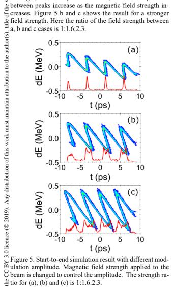
U beam is changed to control the amplitude. The strength ratio for (a), (b) and (c) is 1:1.6:2.3.
