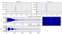
Figure 10: Spectrum of betatron oscillation, turn-by-turn BPMs, and beam image from bending magnet at the resonance point.
