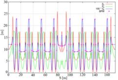
Figure 1: Twiss functions for the double mini-betay lattice in the TPS storage ring.
