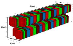
Figure 3: Magnetic model of U114 undulator, modelled by Radia [4].
