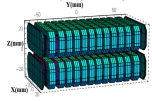
Figure 1: The magnetic model of U18 by Radia code [4].
