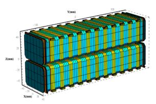
Figure 4: Magnetic model of W44 wiggler, modelled by Radia [4].
