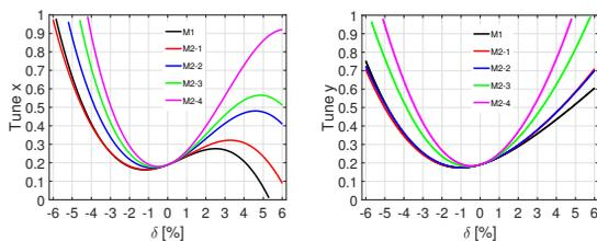
Figure 8: Momentum dependent tune footprints for the four lattices of the second method compared to the M1 lattice.
