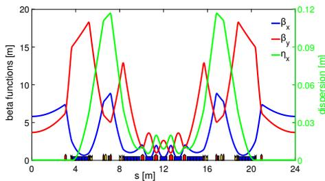
Figure 2: Linear optical functions and magnet layout of the selected lattice. In the magnet layout, bends are in blue, quadrupoles in red, sextupoles in yellow and octupoles in brown.
