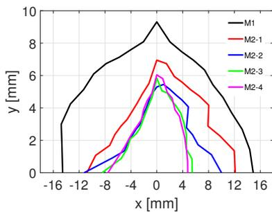
Figure 7: DAs for the four lattices of the second method compared to the M1 lattice.
