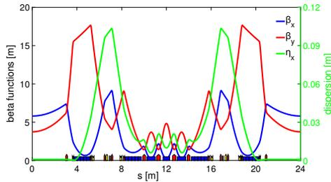
Figure 6: Linear optical functions and magnet layout of the M2-1 lattice.
