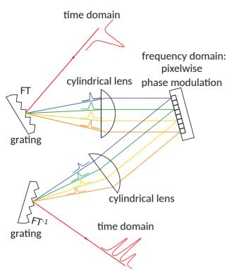
Figure 4: Temporal shaping of a laser pulse is possible by optically mapping the beam onto the Fourier plane and introducing a frequency-selective phase shift. The angles and distances are not to scale.
