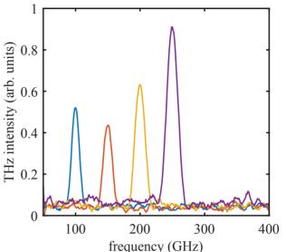
Figure 5: Narrowband sub-THz spectra acquired using a spatial light modulator.
