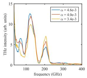
Figure 3: THz spectra measured for slightly different values of the momentum compaction factor  $\alpha$ . The standard operation mode is shown in blue.
