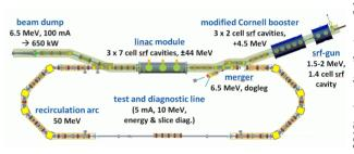
Figure 2: Layout of bERLinPro: The low energy part is highlighted in green.
