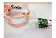
Figure 7: A 40 watts wireless charging module can induce current up to a distance of 5cm.
