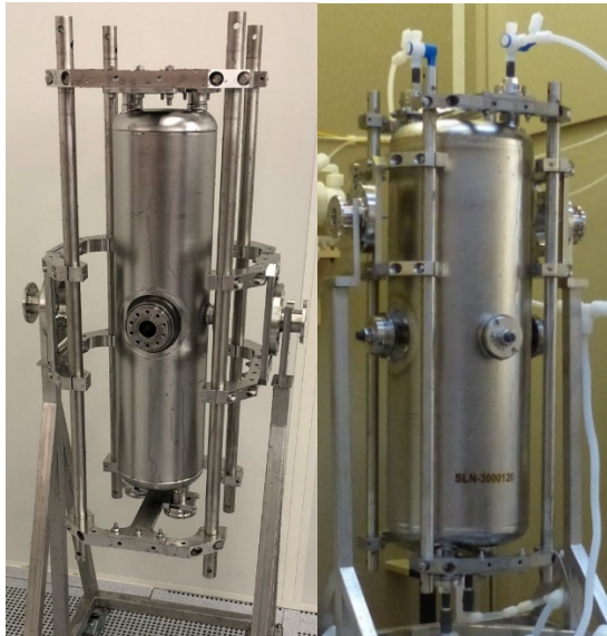
Figure 3: Picture of the low- and high-beta cavities in clean room waiting for assembly and during BCP respectively.
