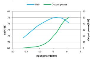
Figure 3: SSPA transmitter output power and gain. Maximum gain is 78 dB at 31 kW and maximum power is 50 kW with a compression of 1.8 dB.
