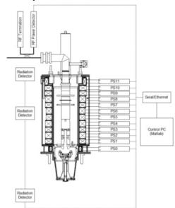
Figure 10: Setup plan for the experimental validation of the beam-loss suppression by optical matching in klystron. The optical matching at various beam sizes is achieved by inserting an iron shim between the gun and the magnet aperture, z-translating the gun, and independently powering the pancake coils of the solenoid magnet.
