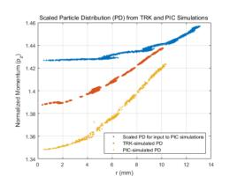
Figure 6: Scaled (top) particle distribution(PD) for input to PIC simulation. It is obtained from the PDs in downstream plane of the TRK (middle) and PIC (bottom) simulations. PIC-simulated PD has larger potential depression than TRK-simulated PD due to unrealistic.
