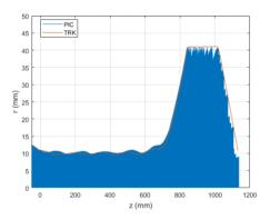
Figure 4: TRK-simulated beam envelope and PIC-simulated beam profile. In the PIC simulation, the injection boundary is at z = -50 mm which is 150-mm downstream from the cathode.
