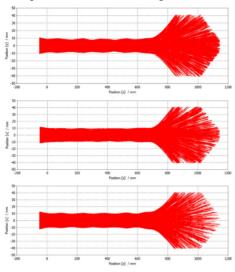
Figure 3: Non-matched (top) and matched (middle) beam profiles simulated by the CST-PIC. Bottom figure shows slightly mismatched beam at larger beam size.
