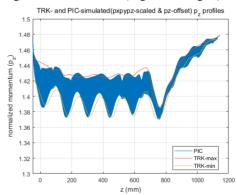
Figure 7: PIC-simulated longitudinal momentum profile with scaled initial PD to match to the TRK-simulated profile.
