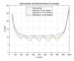
Figure 2: Non-matched and matched beam envelopes simulated by the CST-TRK.
