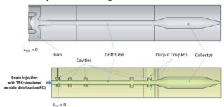
Figure 1: Setups for TRK(up) and PIC(bottom) simulations. Unlike the TRK the PIC does not include the gun into the simulation setup which results in significant errors in beam optics.
