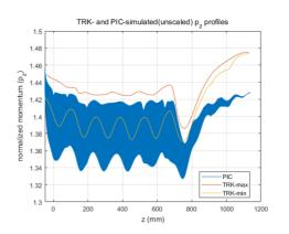
Figure 5: Longitudinal momentum profiles simulated by the TRK and PIC. The PIC profile shows unrealistic potential depression.
