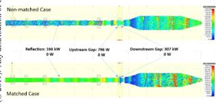
Figure 9: PIC-simulated beam-energy profiles for nonmatched(top) and matched(bottom) beams. With the nonmatched beam there are significant beam losses which are  $\succeq$  successfully suppressed by the matched beam. Simulation condition: Beam voltage = 400 keV, Beam current = 500 A, RF output power = 80 MW, Drive powers are 300 W for the non-matched beam and 75 W for the matched beam. An efficiency improvement of several percent as well as ~6- dB gain increase are attained.
