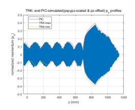
Figure 8: PIC-simulated transverse momentum profile with scaled initial PD to match to the TRK-simulated profile.
