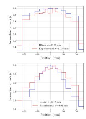
Figure 5: Comparison with experimental results at two positions in the beamline. The red line correspond to the experimental data and the blue line to the results obtained with our model.
