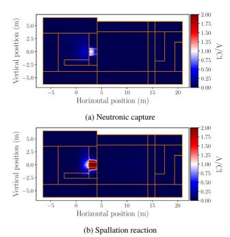
Figure 6: Representation (top view) of the quantity of activated concrete due to neutronic captures in (a) and spallation reactions in (b). The walls are represented by the orange lines.
