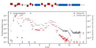
Figure 3: Locations of beam losses along the beamline. They are mainly located at the beginning and near the energy degradation system for an energy at isocenter of 70 MeV.
