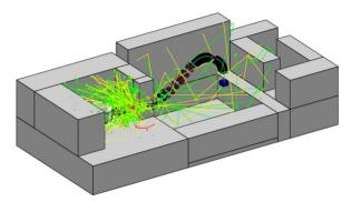
Figure 4: Realistic model of the Proteus<sup>®</sup>One system for BD-SIM simulations combining the shielding and the beamline. The proton beam (cyan) is transported up to the isocenter but produces neutrons and gammas (green and yellow) when interacting mainly with the energy degrader.
