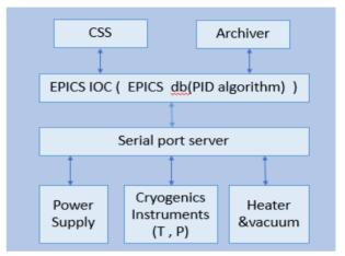
Figure 2: The structure of SCW EPICS control system.
