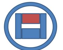
Figure 2: The structure of the cross section of SAU. The horizontal rectangles represent the magnetic pole and magnet of the SAU. The vertical rectangles represent the side magnets outside the SAU, whose magnetization direction is opossite to the solenoid. The outer ring represents the solenoid.
