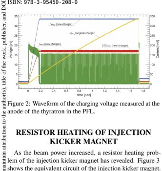
Figure 2: Waveform of the charging voltage measured at the anode of the thyratron in the PFL.
