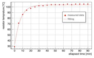
Figure 5: Measured temperature of the resistor for the nominal current and 2.48 sec repetition period.
