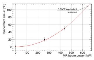
Figure 6: Measured temperature rise of the resistor versus MR beam power.
