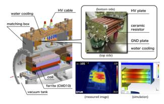
Figure 4: Resistor unit housed in the matching box.
