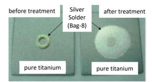
Figure 3: Pictures of the silver solder on the pure titanium surface before and after heat treatment. Outer diameter:  $4.35\phi$ mm(before),  $\sim 11\phi$ mm(after), Inner diameter:  $2.5\phi$ mm(before), 0mm(after).
