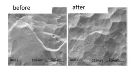
Figure 1: SEM Pictures of surface of the pure titanium before and after nitric hydrofluoric acid treatment.
