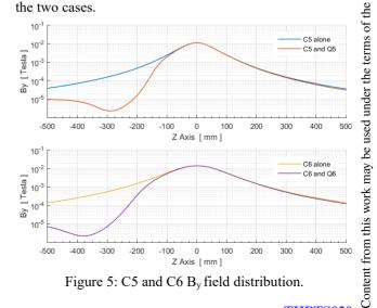
Figure 5: C5 and C6 B<sub>v</sub> field distribution.
