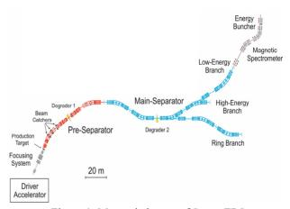
Figure 1: Magnetic layout of Super-FRS.
