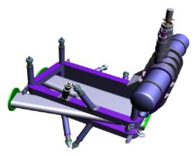
Figure 3: Cryostat and vacuum chamber of the branching dipole. Due to the opening for the chamber the coil casing supports have to be inclined to be able to cope with the magnetic forces.
