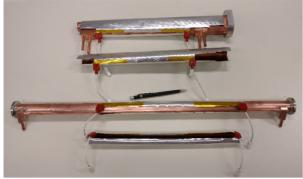
Figure 2: Tapes covering two different shapes of chamber along with the shape-memory after a heating process.
