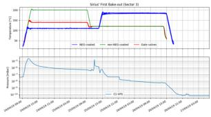
Figure 7: Experimental heating stages of some channels and pressure evolution during the NEG activation of the first achromatic arc installed.
