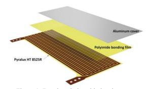
Figure 1: Developed ultra-thin heating tape.
