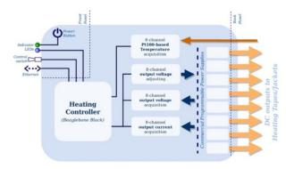
Figure 5: Block diagram of Baking Power Crates.
