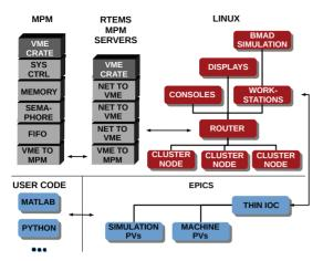
Figure 2: Block diagram showing how our EPICS interface integrates with legacy CESR control and simulation software: clockwise from bottom, user code interacts with both machine and simulation by setting and getting Process Variables (PVs) through the network Channel Access protocol; a thin Input-Output Controller running on a Linux workstation acts as the client of a VMEbus interface to the Multi-Port Memory (MPM) that aggregates machine command and sensor data.
