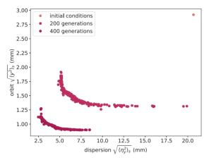
Figure 4: Trade-off frontiers in the space of orbit and dispersion for a misaligned lattice, as found by the Platypus genetic algorithm package driving a BMAD simulation via our interface.
