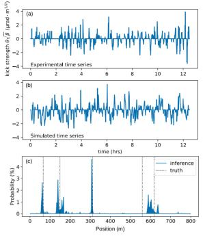
Figure 5: (a) typical kicker strength time series obtained from CESR orbit data; (b) kicker strength fluctuations simulated as an Ornstein-Ulenhbeck process, Eq. (3); (c) histogram of drifting kicker locations as inferred from fits to simulated data.
