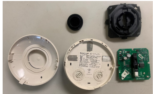
Figure 3: Visual inspection of failed smoke detectors.
