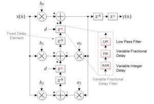
Figure 4: OTFB – Biquad (IIR) with fractional delay FIR filter.
