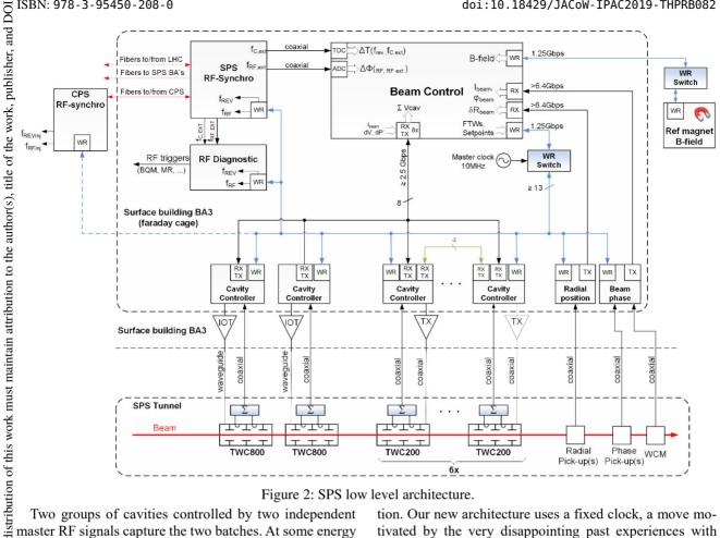
Figure 2: SPS low level architecture.
