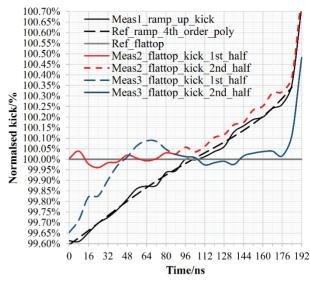
Figure 4: Three measured, normalised, kick waveforms and reference waveforms at  $\pm 5$  kV.
