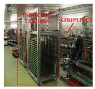
Figure 2: The CLIC DR prototype inductive adders and striplines installed in the ALBA Storage Ring.
