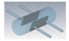
Figure 3: 3D model of the stripline with 4 feedthroughs.
