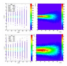
Figure 5: Horizontal beam profile along the longitudinal direction (left) and energy deposition on the x-z plane (right) in the water box for 70 MeV FLASH beam for Method 1 (top) and Method 2 (bottom).
