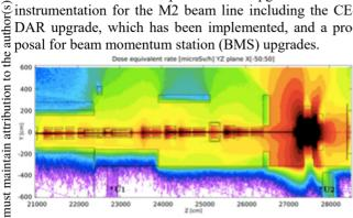
work Figure 8: Preliminary simulation results for the radiation map of the 2018 high intensity hadron beam (3.8 x  $10^{8}$ /spill) at the entrance to EHN2, where the beam is en-· of · tering from the left side.
