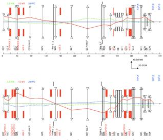
Figure 2: Tentative optics for a parallel beam for the upstream located experiment with a focused beam downstream.
