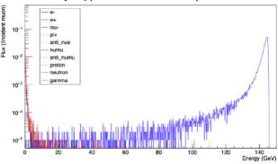
Figure 5: Produced particles after passing MuonE (FLUKA / Geant4).
