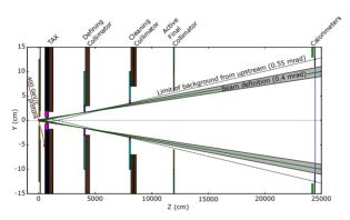
Figure 2: Layout of the K12 beamline for KLEVER, with the four-collimator system for selecting the neutral beam.
