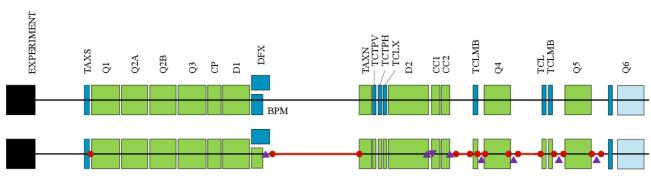
Figure 1: Side view of an HL-LHC high-luminosity IP with quadrupoles (Q), corrector package (CP), dipoles (D), collimators and masks (TC), crab cavities (CC), absorbers (TAX), deformable RF bridges (red circles), fixed beam pipe sections (red lines) and sector valves (purple triangles): HL-LHC Technical Design Report (top) and FRA Study (bottom).
