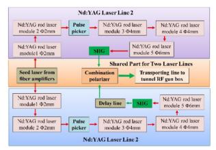
Figure 2: Configuration of the Nd:YAG rod laser amplification part of the current laser system.
