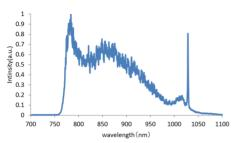
Figure 3: Spectrum band of supercontinuum light obtained from Yb doped fiber.
