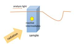
Figure 1: Scheme of the pulse radiolysis system.
