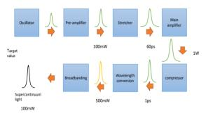
Figure 4: The procedure of supercontinuum light generation. The values in the figure show the target average power and pulse width at each stage.
