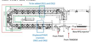
Figure 1: New ALPI layout with highlights on the position of the new cryostats (in blue) and higher gradient triplets (in green). Injection from stable beams (Tandem and PIAVE) and exotic ones (SPES new RFQ injector), and the direction of the beam are marked by red arrows.
