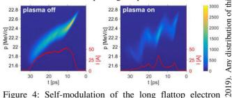
Figure 4: Self-modulation of the long flattop electron bunch passing through a plasma. Bunch momentum and transverse distribution are modulated, as seen in the LPS and the charge profile. The bunch head is on the right.
