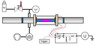
Figure 3: Concept sketch of the PITZ gas discharge plasma source. Source: [12].
