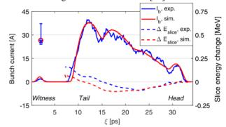
Figure 5: Measured and simulated bunch current profiles (solid lines) and deceleration within the driver bunch (dashed lines). Blue cross and red circle represent the maximum energy gain within the witness in the experiment and simulation, respectively. Source: [22].
