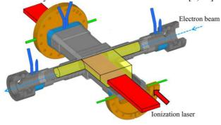
Figure 2: Concept sketch of the PITZ heat pipe oven plasma source.
