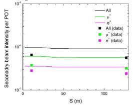
Figure 5: Simulated performance along the M4 and M5 lines. The squares indicate the measured intensity at the entrance and exit of the lines for the different species.
