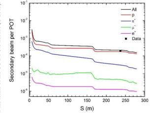
Figure 2: Simulated performance of the transmission of secondary particles. Plots for different acceptances are shown.
