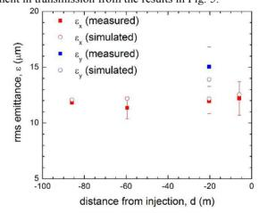
Figure 6: Emittance along the final stretch of the M5 line. Note that d=0 denotes the entrance of the storage ring.
