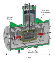
Figure 1: Sectional view of Demonstrator cryostat, the 216.816 MHz CH-cavity and two sc solenoids are suspended within a support frame.
