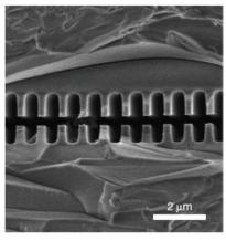
Figure 4: Scanning electron microscope image of the longitudinal cross-section of a DLA structure [14].
