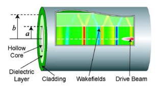
Figure 3: Conceptual drawing of the dielectric wakefield accelerator (DWA) [12],  $a = 50 \mu m$ ,  $b = 162 \mu m$ .
