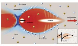
Figure 5: Conceptual drawing of the plasma wakefield accelerator [16].
