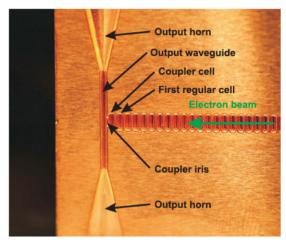
Figure 2: The mm-wave traveling wave accelerating structure with detail of the output part, including coupler and output waveguides [8].
